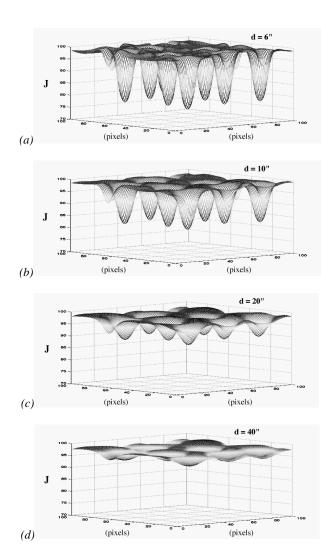
Figure 7. Samples of images in the perceived lightness with cyan dye concentration of 20% viewed at distances of 6", 10", 20", and 40", respectively.
