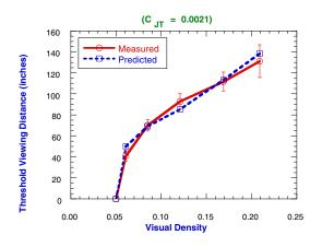
Figure 8. Comparison between predicted and measured threshold distances for samples from the printer. The error bars denote variations over one standard deviation.
