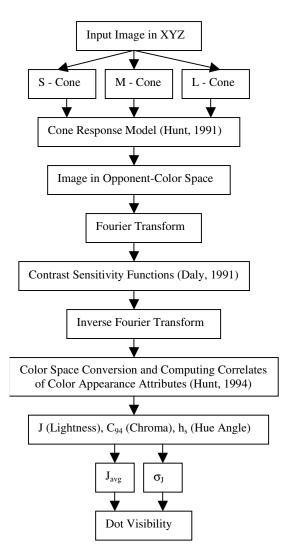
Figure 2. Flow chart of the simplified CVDP for dot visibility prediction.
