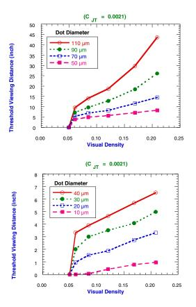
Figure 9. Model predicted threshold viewing distance as a function of dot diameter and visual density.
