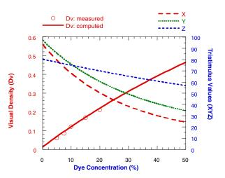
Figure 5. Variations of the measured and computed visual density values and computed tristimulus values with cyan dye concentration.
