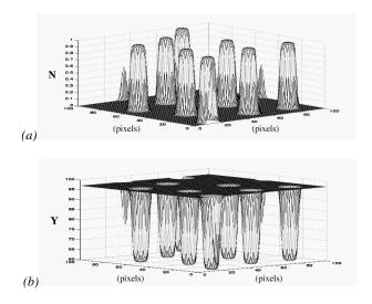
Figure 6. Samples of images in (a) normalized pixel value with dot diameter of 461  $\mu$ m and (b) tristimulus Y value at dye concentration of 20 %.
