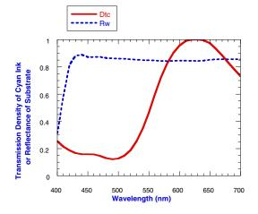
Figure 4. Spectral transmission density of the cyan ink and spectral reflectance of the substrate.
